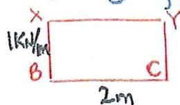
$$\text{Load} = \text{Area } \square BCY \\ = 2 \times 1 = 2 \text{ kN, which} \\ \text{acts through centroid of } \square$$
