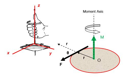
The direction of the moment M is given by the right-hand rule (see diagram above left). Curling the right hand fingers from r toward F (r cross F) gives an upward-pointing thumb which is perpendicular to the plane containing r and F.
